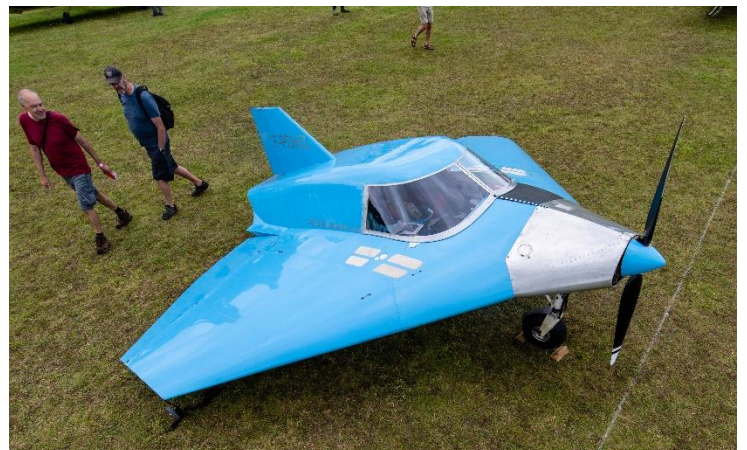
A Rotax 912S-powered Verhees D2 Delta will cruise at 120kt for 7 hours with reserves, plus it's big enough inside to sleep in
